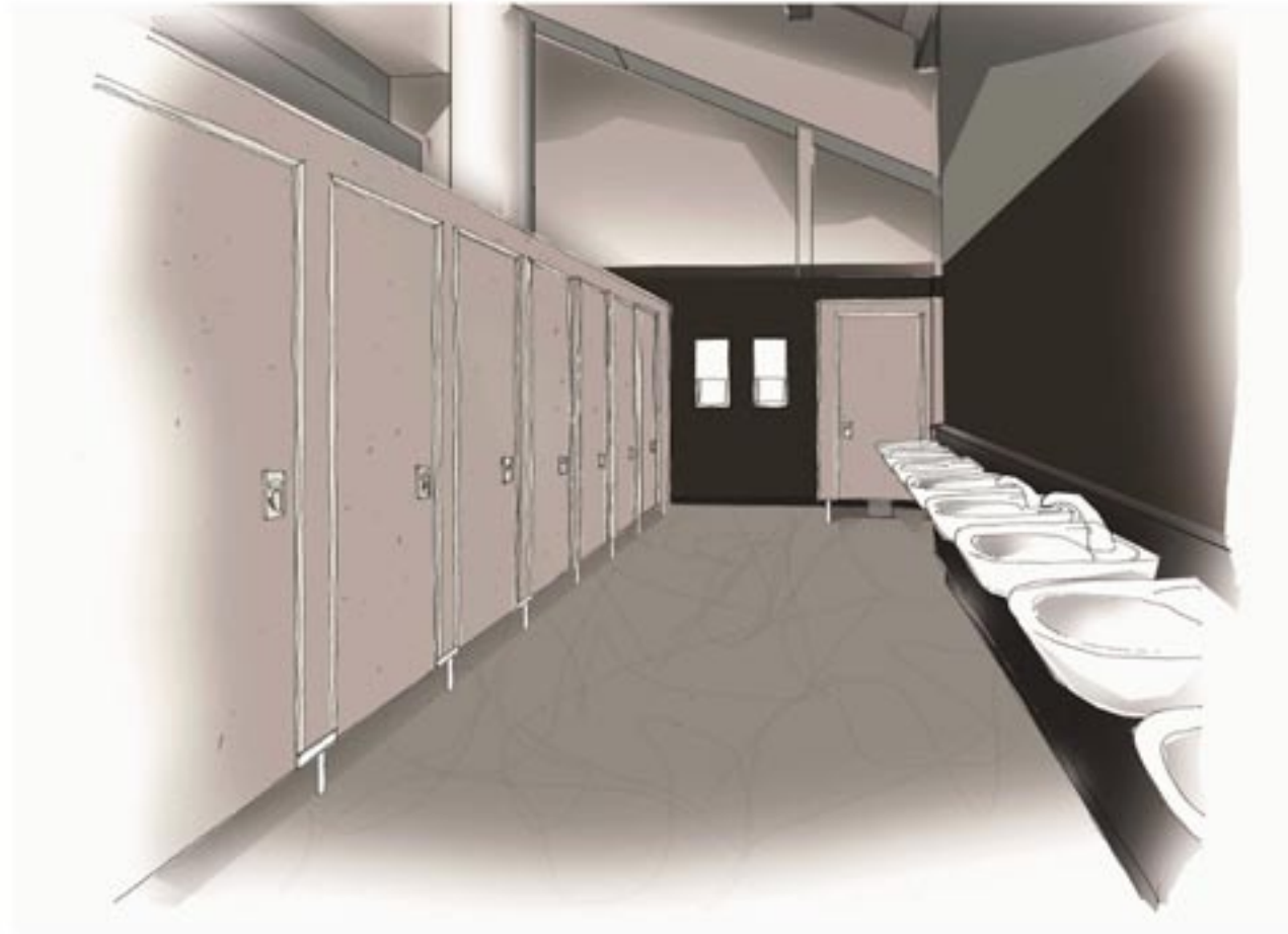
Otago Stadium GA Toilets: Compact laminate toilet partitioning system in aluminium frame. Painted block walls. No ceiling, suspended lighting and other services. Lined false wall behind basins to conceal services. Ceramic basins. Stainless steel trough urinal.
