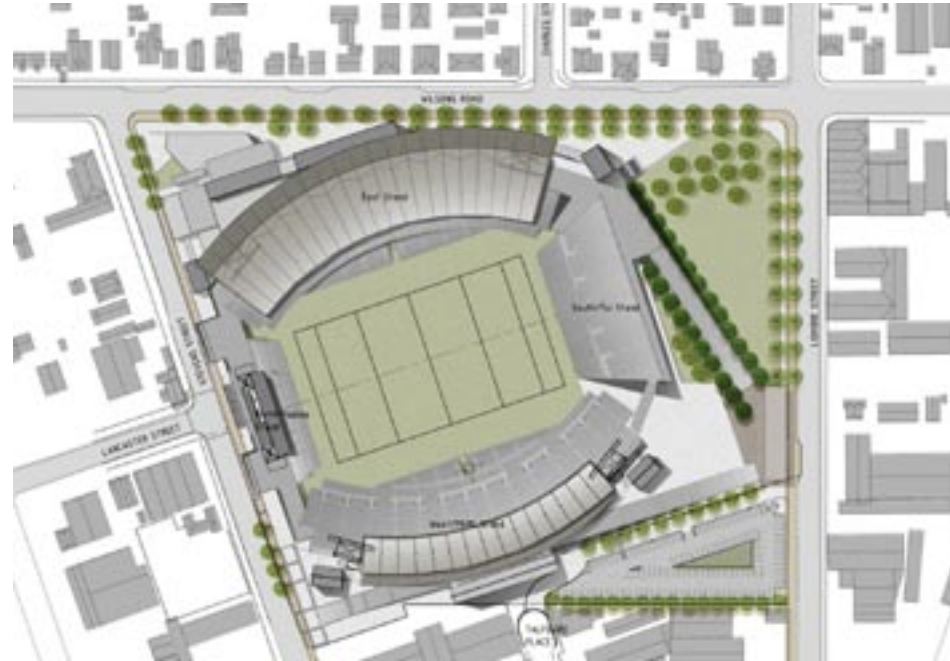
AMI Landscaping: Combination asphalt and paved surfaces, planted tree avenues and green space. Paving includes exposed aggregate paver feature strips and asphalt to pedestrian areas.
