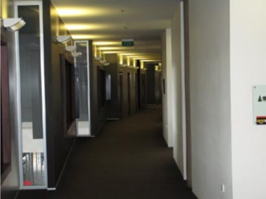
AMI corporate corridor: Painted plasterboard feature wall, with aluminium skirting, wall mounted up lighting, plaster board ceiling
