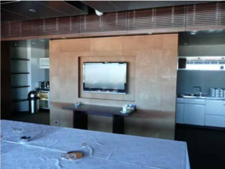
AMI Founders Lounge: Stone feature wall, recessed niche for TV. Batten screen along ceiling edge to kitchen. Kitchen joinery white LPL with ply shelving and mirror backed shelving units over.
