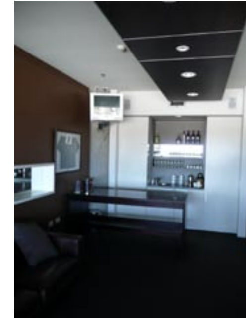
AMI corporate box: Integrated joinery unit LPL, flanking full height cupboards with central formica servery, shelving unit with incandescent down light in bulkhead above. Broadloom carpet. Timber veneer door with timber frames.
