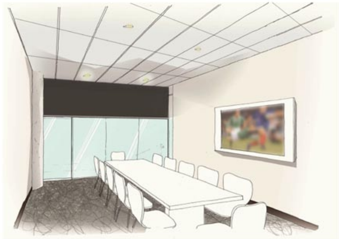
Otago Stadium Corporate Box: Suspended mineral tile ceiling, Recessed downlights. No bulkheads or other features. Painted plaster board walls with timber skirting. Framed shop front glazing with single hinged door, height 2.7M. Glass returns every second wall. No exterior soffit treatment
