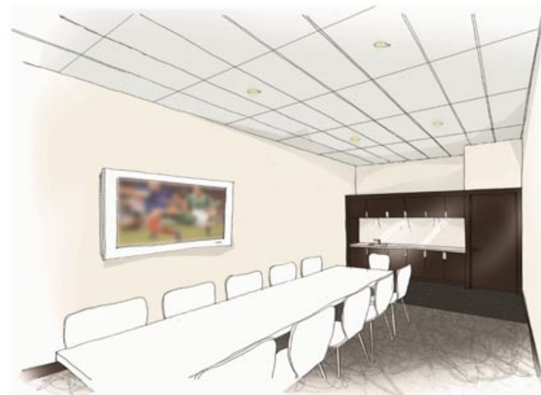
Otago Stadium Corporate Box: Integrated joinery unit, cupboards under and over, 3 recessed halogen down lights. Laminate door and frames. Vinyl floor strip across servery with carpet tiles generally
