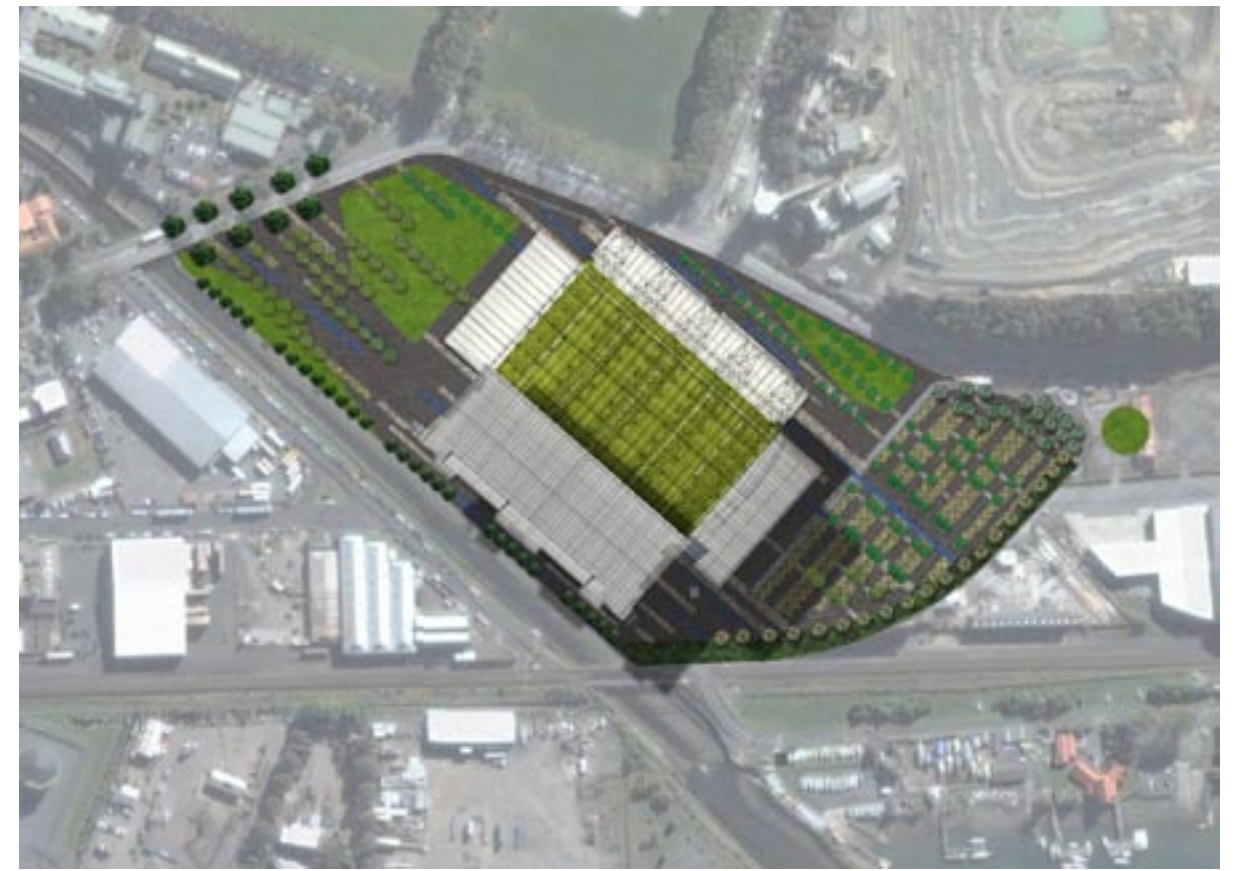
Otago Stadium Landscaping: Combination of asphalt and painted asphalt with concrete paving. Planted areas to car parking and plazas.
