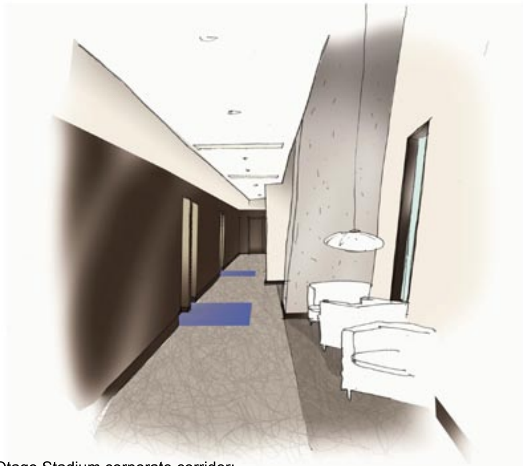
Otago Stadium corporate corridor: Feature paint dado to plaster board lined wall with timber skirtings, stained timber window jamb liners. Carpet tiles in 3 colours. Plaster board bulkhead ceiling, recessed downlights and fluorescent strips. Pendant lights to side.
