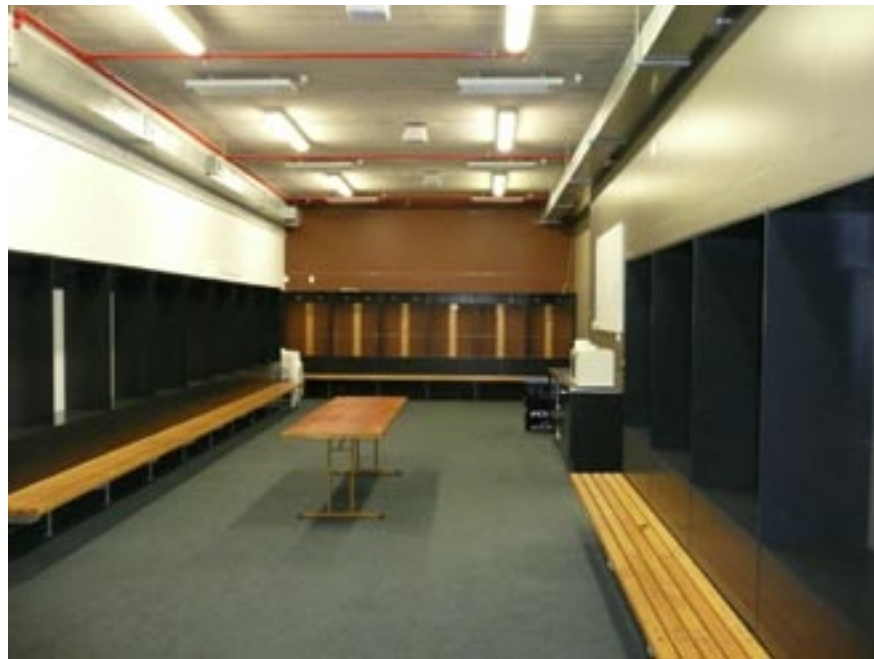
AMI Players Change: Painted plaster board walls. Spray lacquer joinery with foot locker, 2 hooks, partition and shelf and timber bench. Memorial name plates to home team area. Rubberised flooring with skirting. No ceilings
