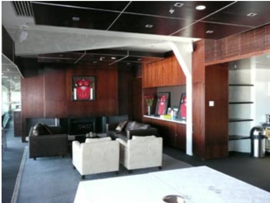
AMI Founders Lounge: Exposed concrete structure plywood wall panelling and joinery units, plywood feature ceiling with recessed down lights. Frameless glass doors with bi-folding leaves 2.4 M high. Broadloom carpet.
