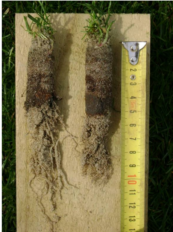
Figure 10. Soil cores for root analysis taken from the control plot in the uncovered area (left) and the control plot in the ETFE covered area (right) three months after the ETFE test rig was installed. Root mass in the 50-100 mm section was not significantly greater from the uncovered area but a root growth differential between the two trial areas was seen to be emerging.
