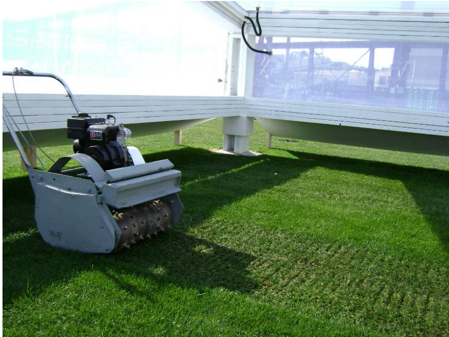
Figure 2. Artificial wear application machine – a modified petrol powered 20" Lawn Master mower fitted with studded rollers rotating at slightly different speeds. Extra weights were fitted on the front of the machine to increase grass-wearing effectiveness.
