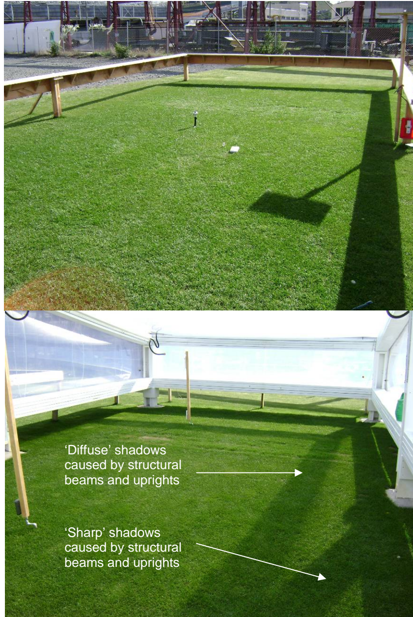
Figure 5. Light conditions at 10:00 NZDT on 10/10/07 showing the difference between 'sharp' and 'diffuse' shadows in the ETFE test rig (bottom photo). The outside test area is shown in the top photo.
