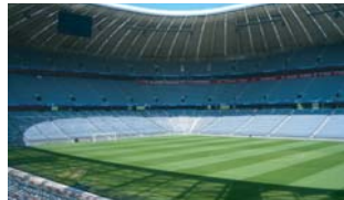
Fig 2.3.8.E-Allianz Arena, DE Complicate heavy shadow on the field of play. When blinds are closed then the transition between light and dark greatly increases and can cause lens flare.
