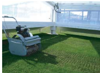
Fig. 2.3.11.B Artificial wear application machine.
