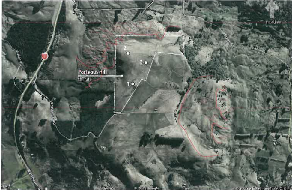
Figure 3: Aerial photograph of the proposed turbine sites with red annotations indicating typical topographic expression of landslides. Solid red lines are 'headscarps' - ie. the upslope limit of the slides; scallops indicate 'hummocky topography' typical of the slumped soil that has separated from the headscarp and slid downhill.
