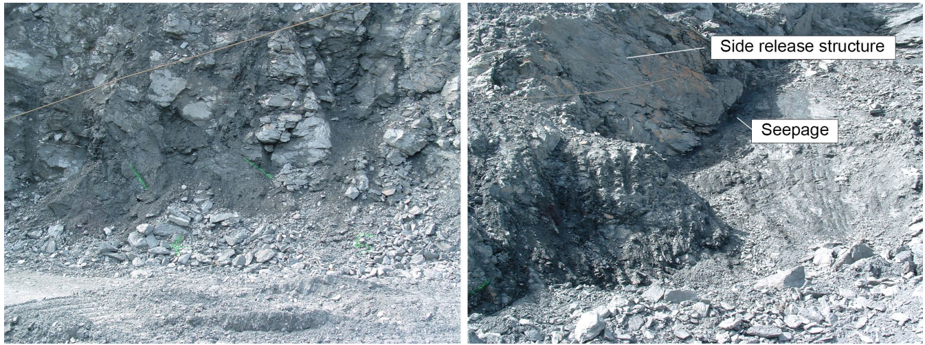
Photo 4: Structural controls of east wall failure. Left: cross-cutting structures in rock mass near failure. Right: northern flank of failure showing side release structure and seepage.
