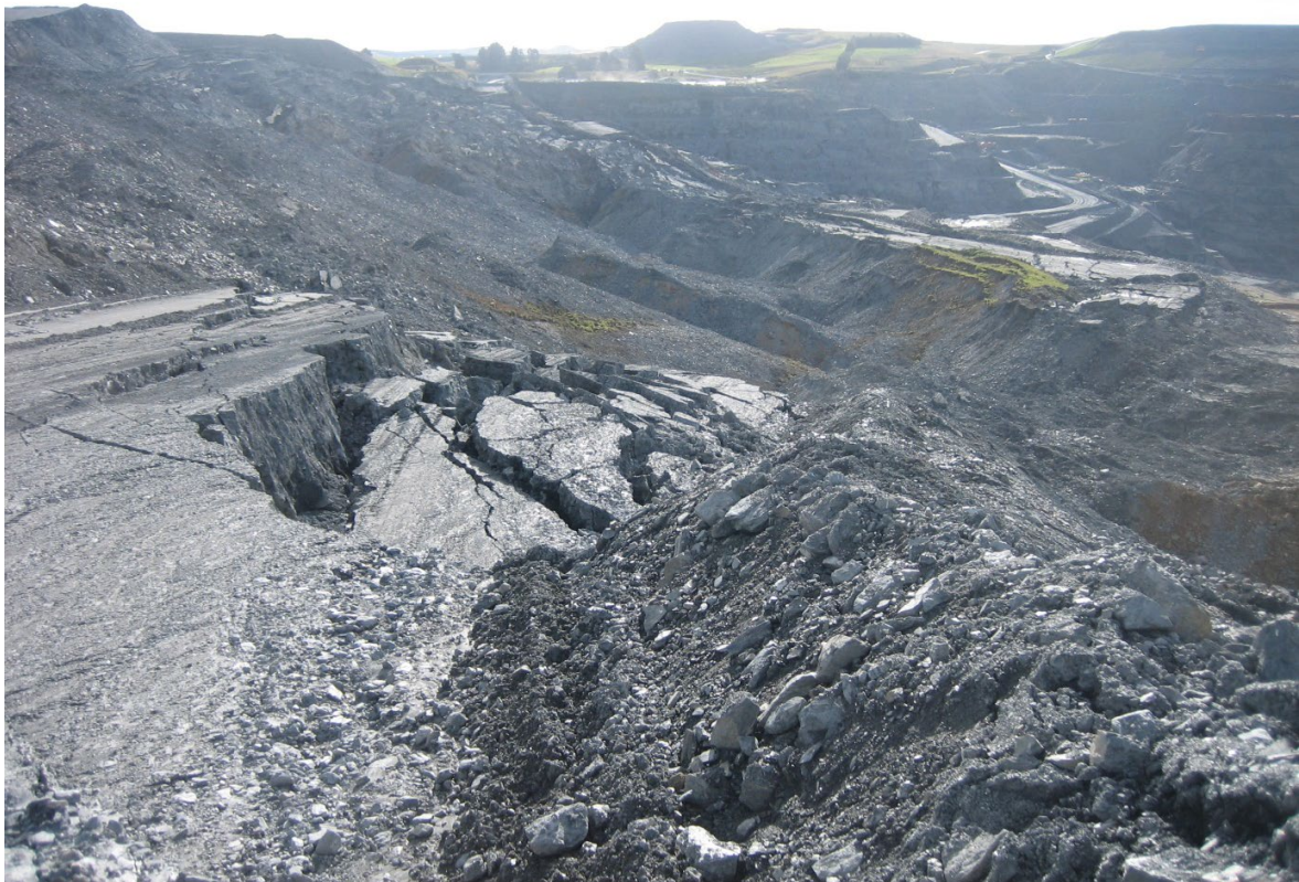
Photo 7: Headscarp of FF exposed at the top of failure. Photo taken along strike towards the north.
