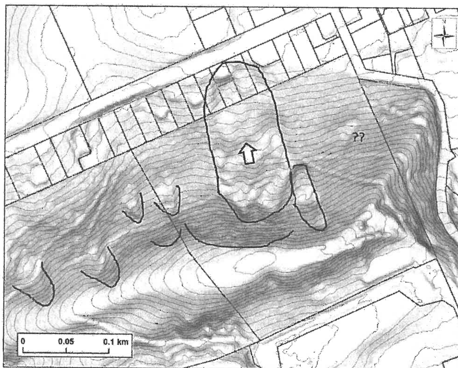
Figure 2. Mapped landslide feature by McKellar (1990) at 82 Riccarton Road East. Other small landslide scarps outlined.
