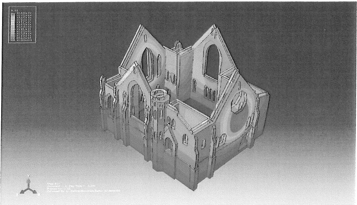
Figure 2.1 This figure shows the magnitude of deflections when the earthquake effects are in the X direction.
