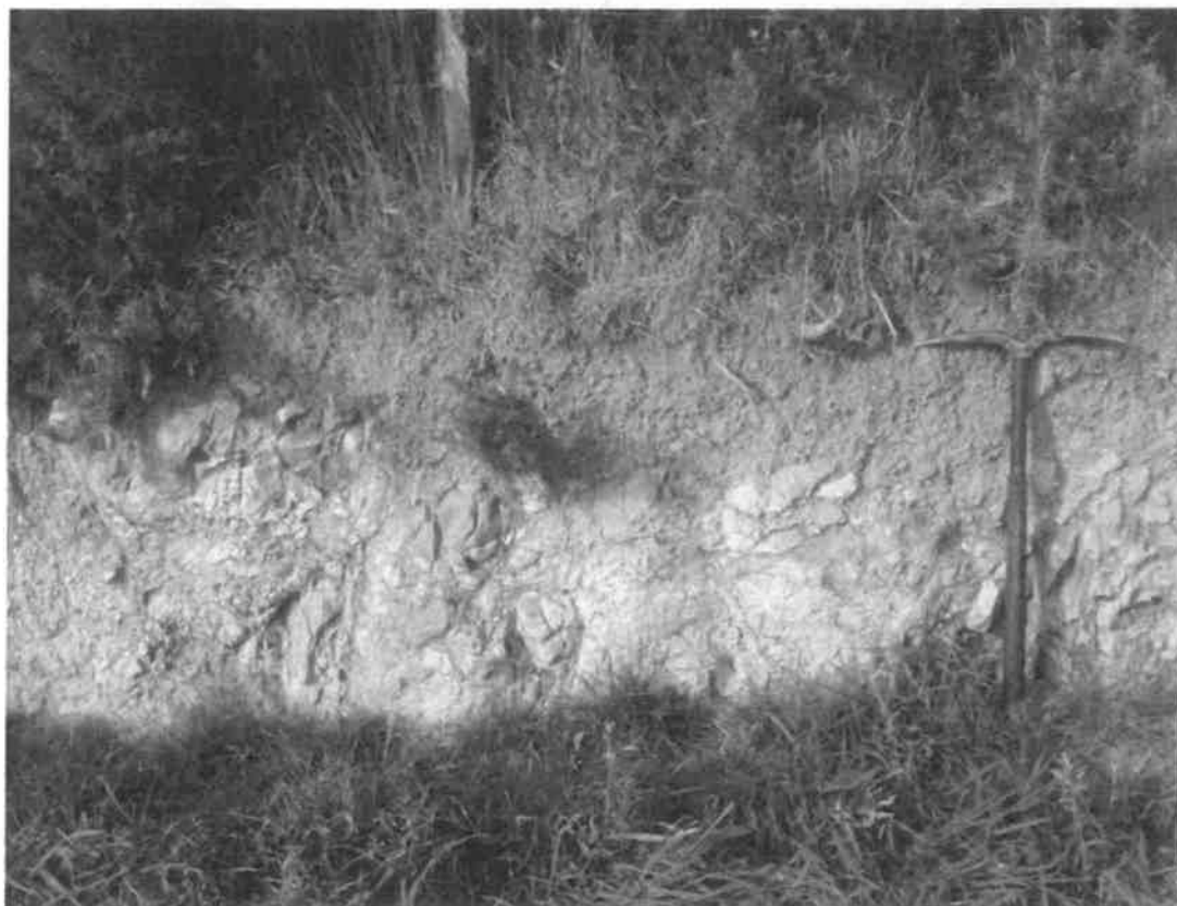
Figure 7 Partially weathered basalt covered by 20-30 cm of top soil, location near vehicle, middle of Fig. 3.
