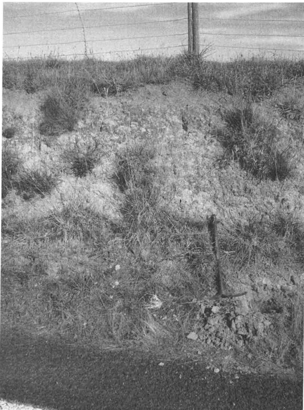
Figure 3 Geological profile exposed south side of Saddle Hill Road, 150 m west of the proposed subdivision, comprises: topsoil and transition zone (30 cm), clayey silt loess subsoil (1.6 m), underlain by strongly leached sandy schist (beneath pick-head). Pick is 85 cm high.
