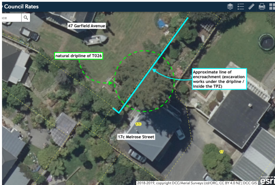
Image four: Image of T026 showing the approximate line and extent of the excavation/soil removal works
