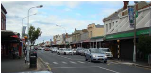
Kerb build outs at pedestrian crossings make crossing easier and safer. However observations suggest that shoppers often opt for the convenience of crossing where they need to, in spite of the increased risks.
