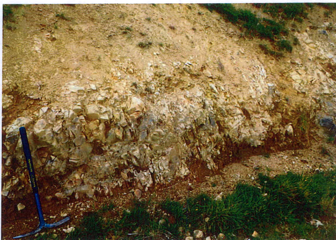
Figure 6 Fresh to moderately weathered jointed basalt exposed in a farm road; left foreground of Fig 3.
