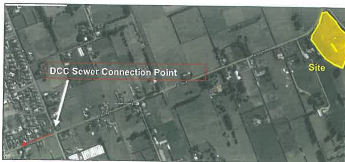
Figure 3.3.1: Sewer Connection Location
