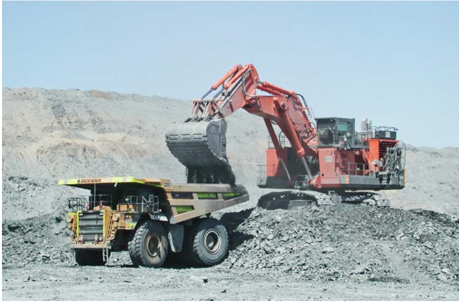
Figure 6. HitachiEX3600 Excavator Loading a Cat 789C Dump Truck
