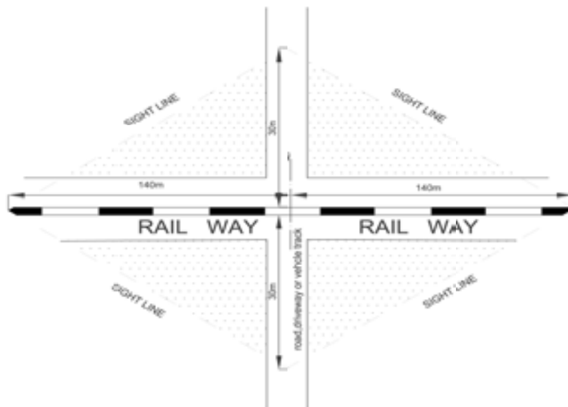
Figure 6B.18 Railway level crossing sight line restrictions
