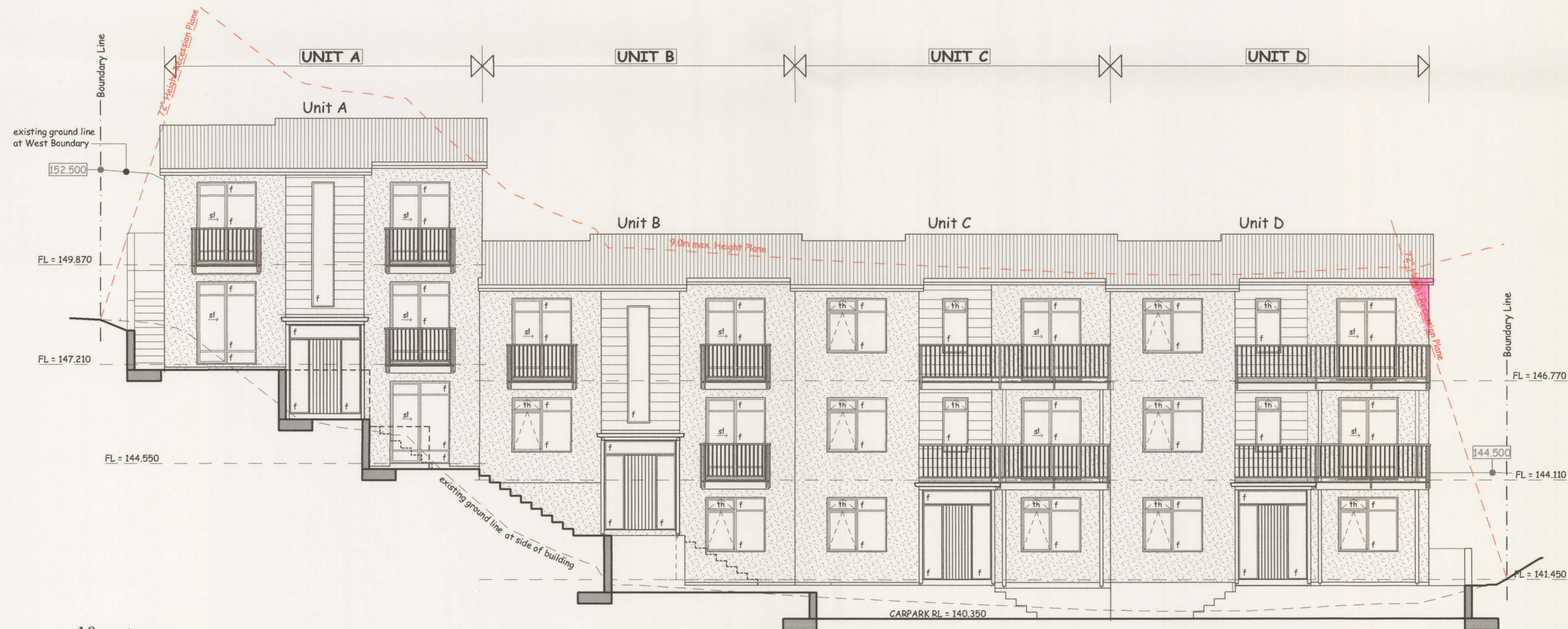
UNITS A/B/C/D - SOUTH ELEVATION 1:100
