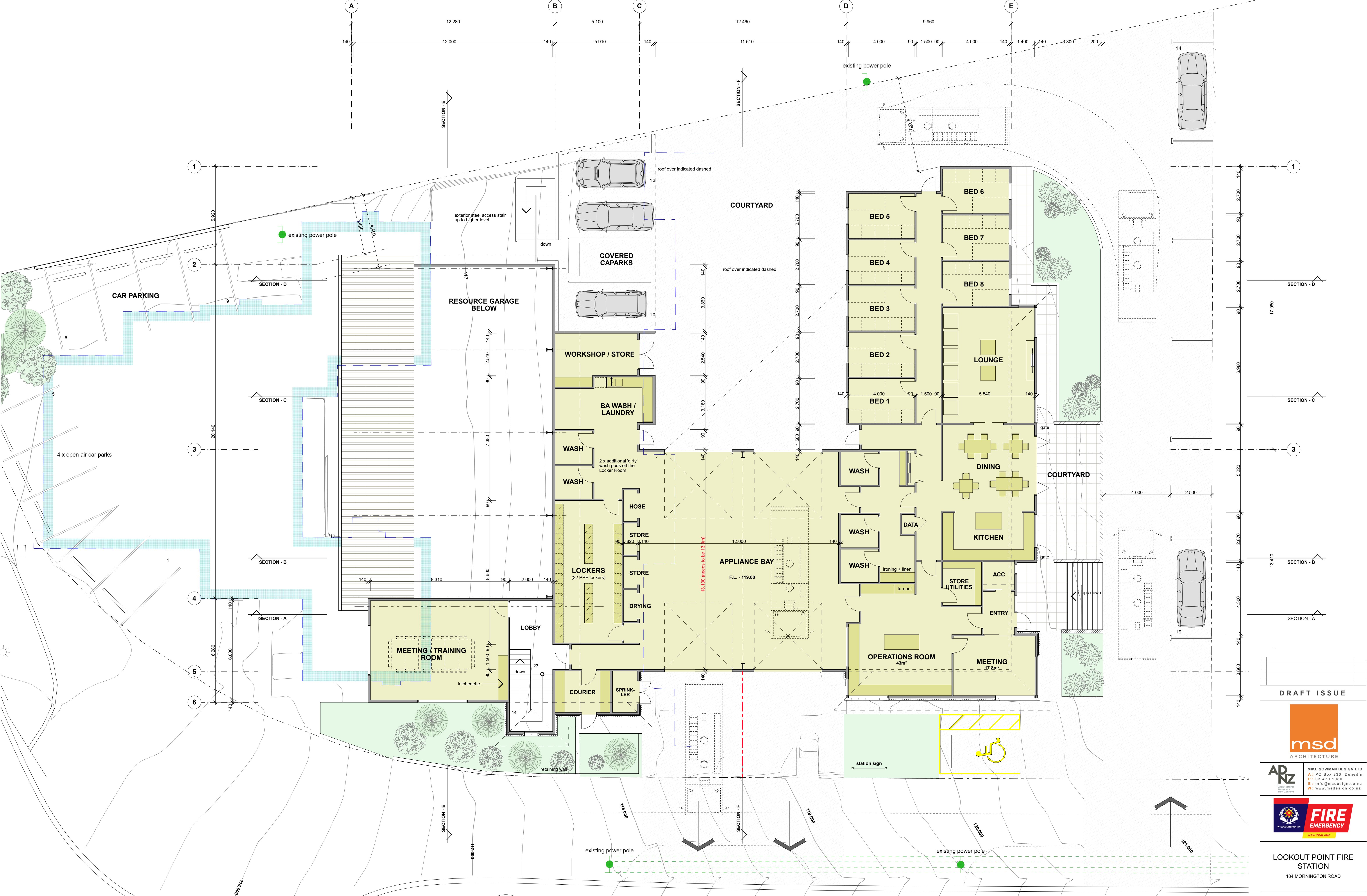
PROPOSED UPPER FLOOR PLAN SCALE 1:100 TOTAL FLOOR AREA = 715m 2
