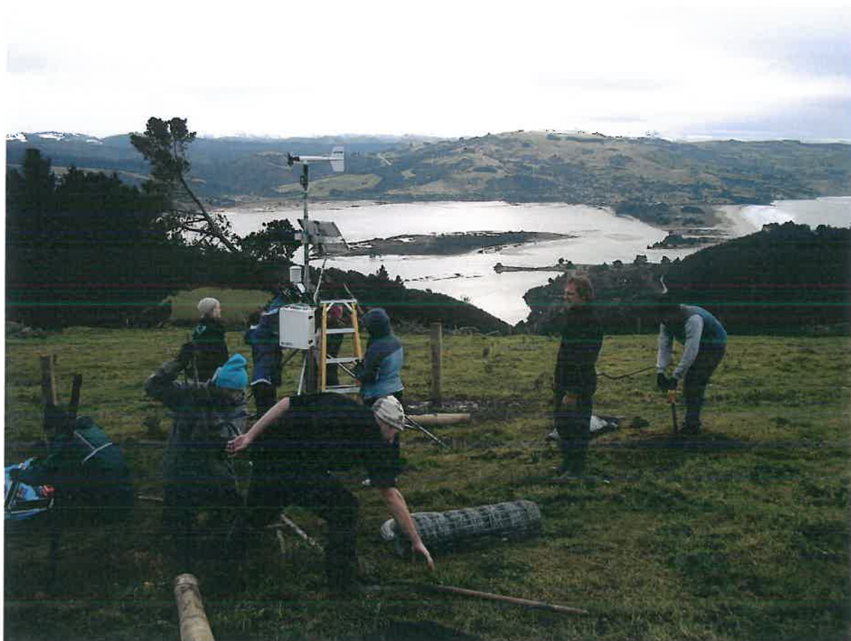
Nicolas Cullen and Geog380 installing Automatic Weather Station 1 on Mopanui Ridgeline above Blueskin Bay, May 2009. Carl Scott/WEP stockphoto, 2009
