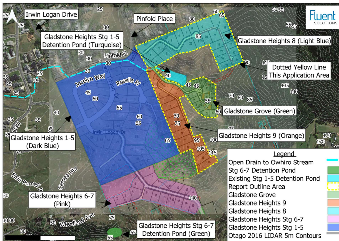
Figure 5.1: Existing Stormwater Infrastructure and Surrounding Catchment
