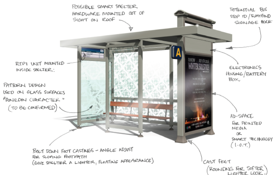
Figure 6 – Dunedin Bus Hub Concept Shelter with Technology
