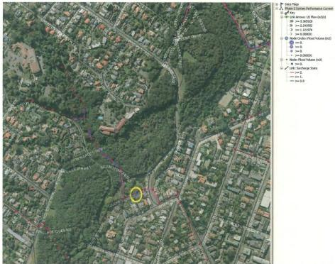
Sewers highlighted in purple are surcharge by depth (a result of downstream incapacity)
