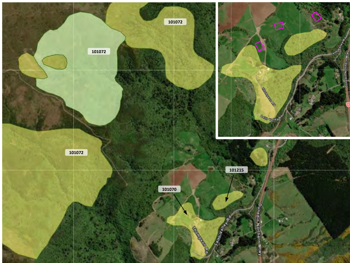
Figure 4. ORC Natural Hazards Database landslide mapping excerpt showing the landslides on the subject site and on the hills to the north and west. Inset shows the landslides on the site in more detail, and the approximate location of the building platforms on Lots 5, 6 and RT OT15B/131 (left to right) (retrieved 30 May 2023).
