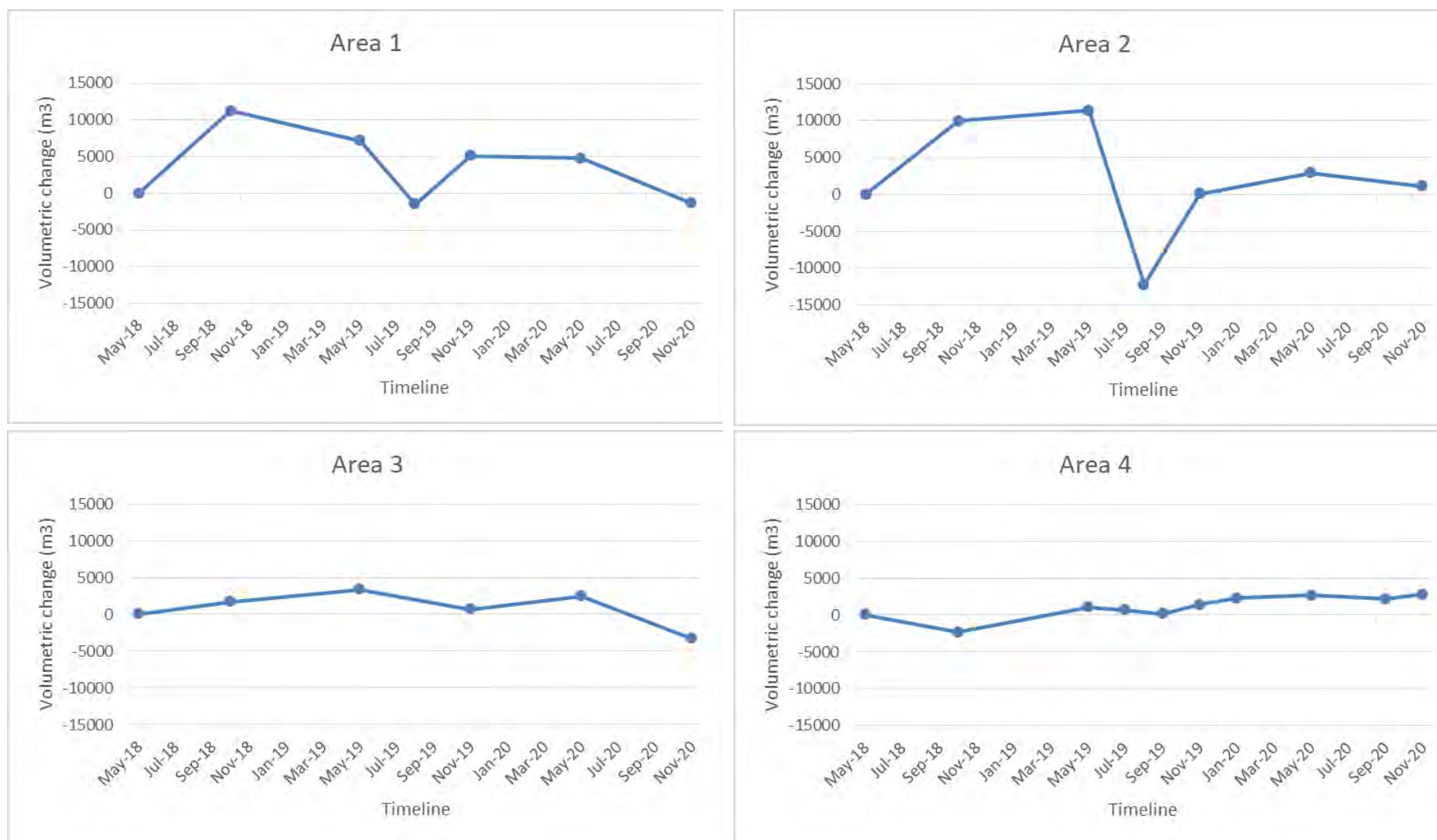
Figure 5.37: Time-series of volumetric sand change in 4 survey areas between the 29 th May 2018 and the 11 th November 2020.
