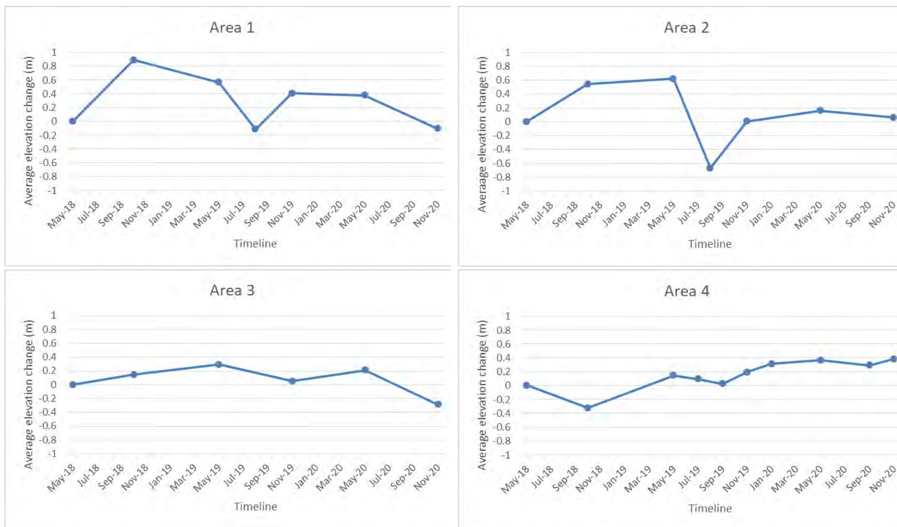
Figure 5.38: Time-series of beach elevation change in 4 survey areas between the 29 th May 2018 and the 11 th November 2020.
