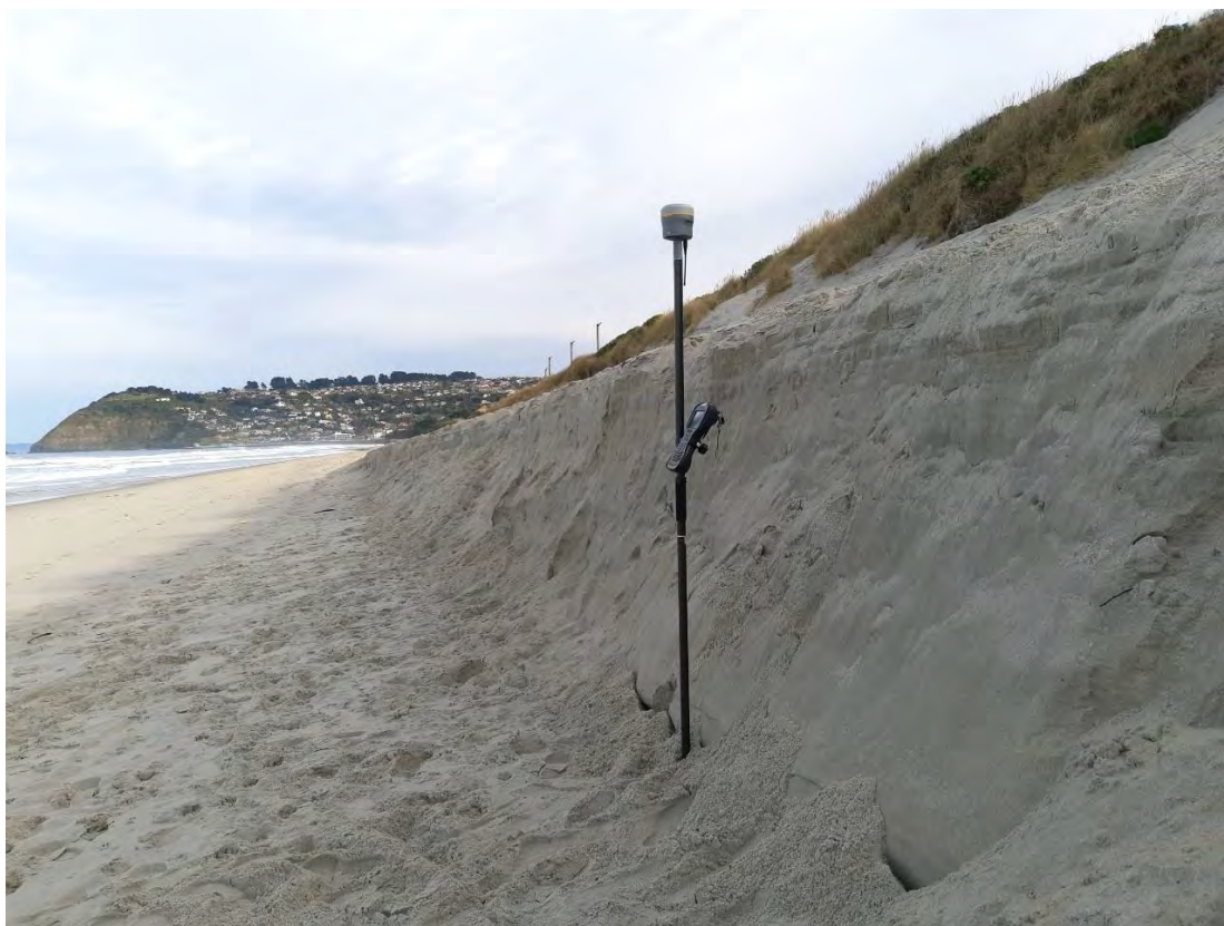
Figure 7.4: Upper beach erosion of approximately 2 m in Area 2 on the 26 th July 2020.
