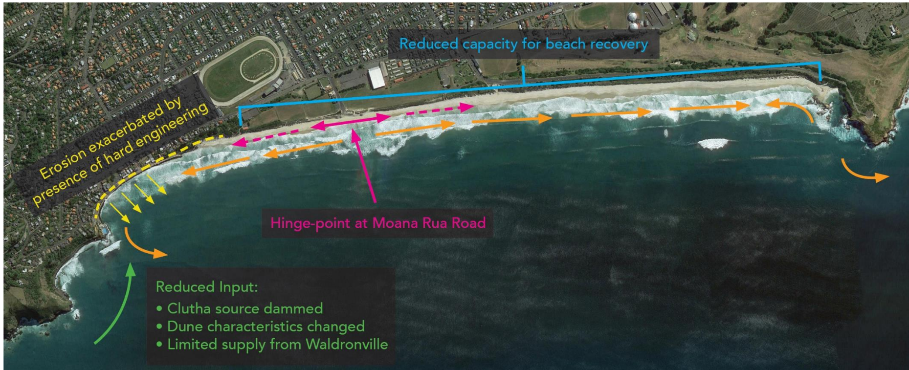
Figure 2: Schematic of process and environmental setting within the St Clair to St Kilda embayment. The Moana Rua Road area is a hinge-point with sediment being transported away from this point in both directions. The Moana Rua Road area is likely the most vulnerable part of the beach and will likely be the first area affected by a sediment deficit. Erosion is very apparent in this part of the beach and it is only ~600 m from the hard engineering at the St Clair end of the beach.
