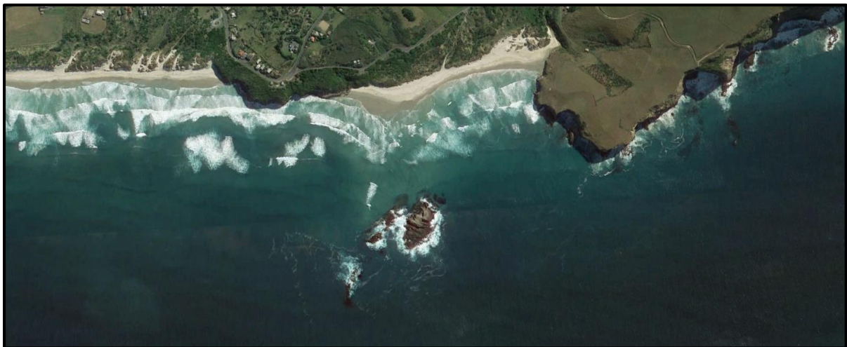
Figure 3: A substantial salient, that is a widening of the beach, is present at Smalls Beach due to Bird Rock just offshore, which reduces wave energy at the beach and rotates waves to reduce LST.
