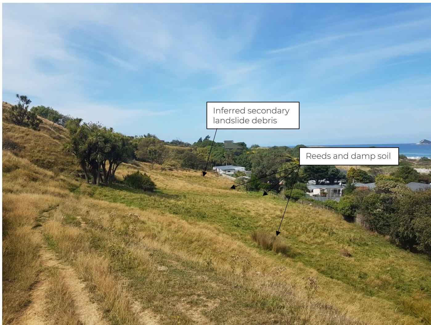
Figure 9: A number of damp areas at the toe of the primary and secondary landslides.
