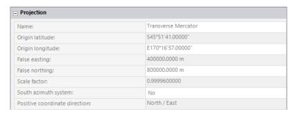
Figure 4: Projection settings to be maintained.
