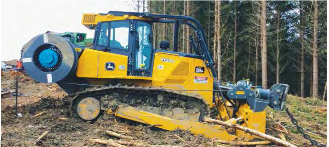
A new ROB – Remote Operated Bulldozer – a tether machine used to assist felling machines when working on steep slopes. It is owned and operated by Gamble Forest Harvesting, contracted to City Forests
