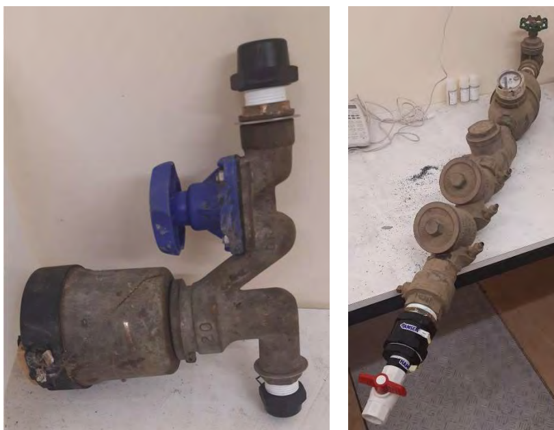
Figure 25: The meter and toby from Karitane Bowling Club (left) and the meter and double check valve with associated fittings and fixtures from Waikouaiti Golf Club (right)
