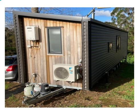
In this example, no services are connected to the ground. The heat pump and water heater are mounted onboard. The unit has a chassis and trailer features that are fit for purpose, including a draw bar length that allows it to be towed away behind a vehicle on the road with relative ease. No permanent services are connected. In this case the tiny home is a moveable vehicle and therefore not a building. **Building consent is not required**.
