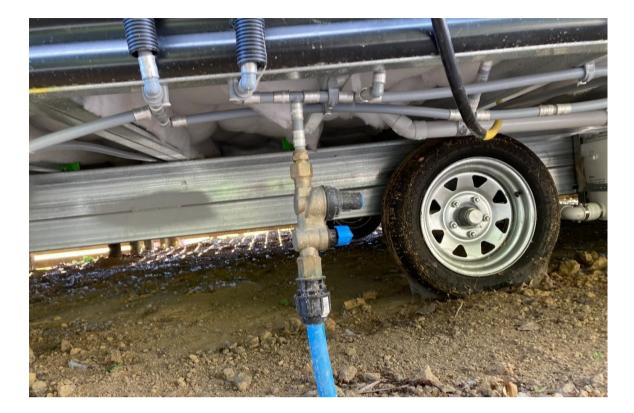
This is an example of a water connection that can be easily isolated and disconnected.
