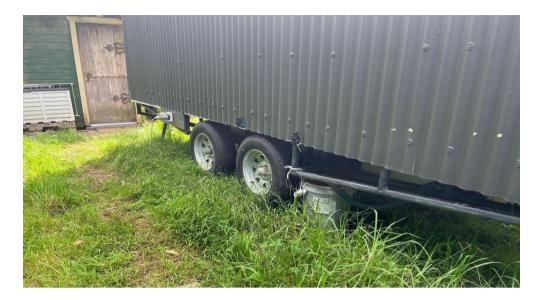
The unit has a chassis, and trailer features that are fit for purpose and allow it to be towed away behind a vehicle on the road with relative ease. The power supply lead is easily removable. No permanent services are connected.
