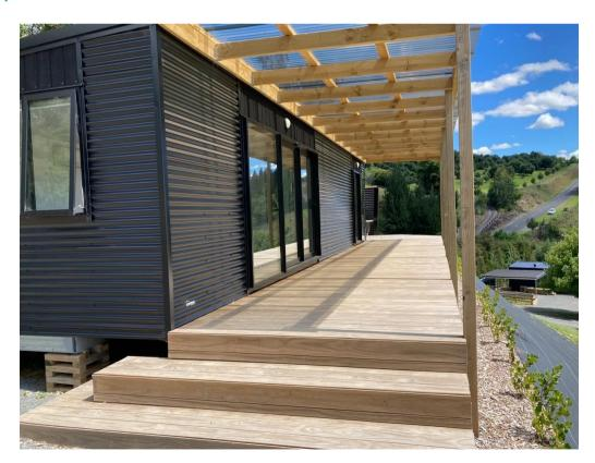
This tiny home is a vehicle with trailer features but is not moveable due to the attached veranda roof. It may be considered to be a building if occupied by people on a permanent or long-term basis and **building consent is required**.
