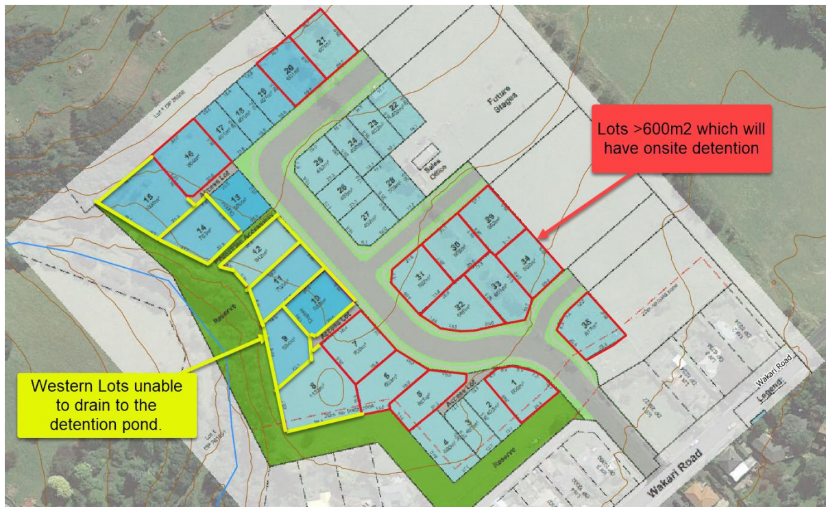
Figure 7.3: Stage 1 Lots with Onsite Detention Tanks
