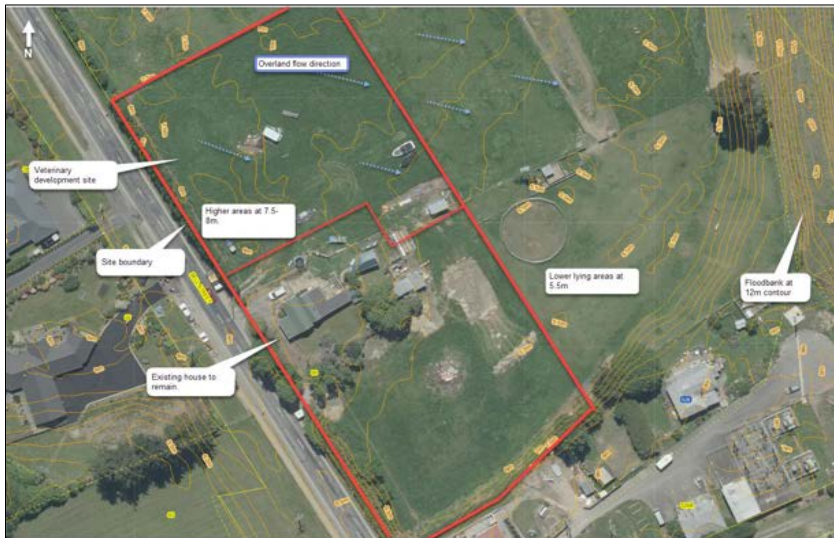
Figure 7: Site Contours and Flood Bank
