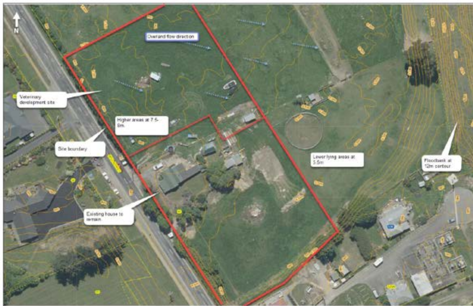
Figure 7: Site Contours and Flood Bank
