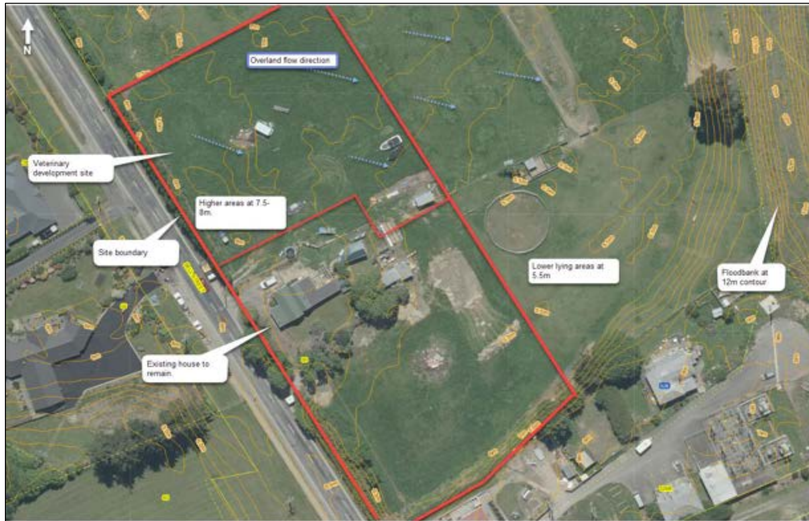
Figure 7: Site Contours and Flood Bank
