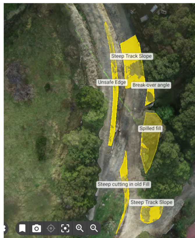
Figure 2: drone image with labels showing 2022 earthworks
