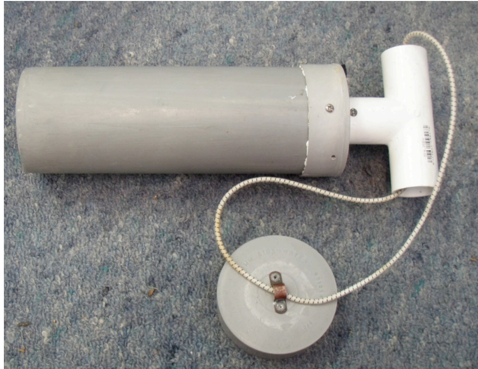
Figure 4. Core sampler used during offshore sampling.
