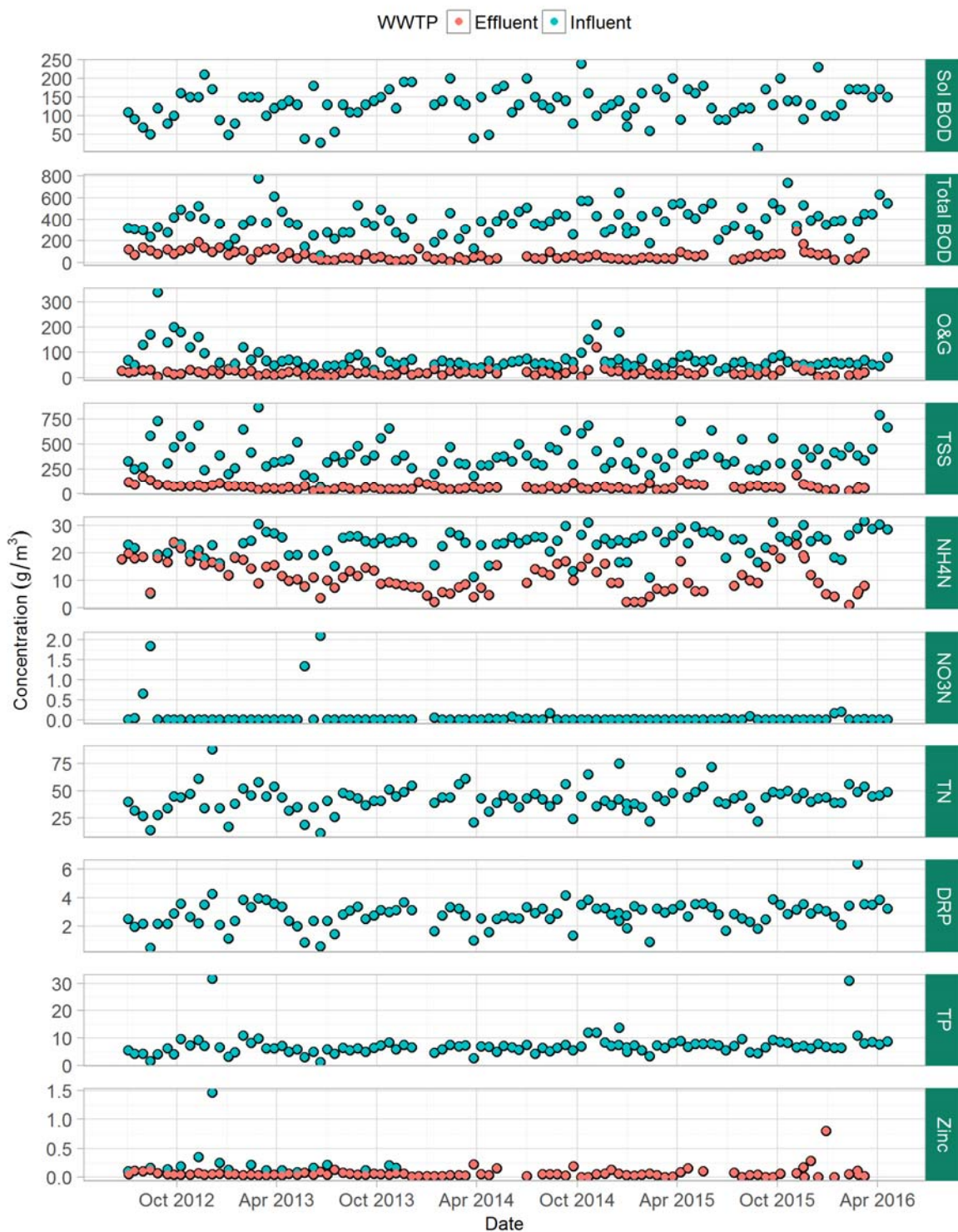
Figure 1: Summary of influent and effluent data for WWTP from 2012 (some outliers excluded).
