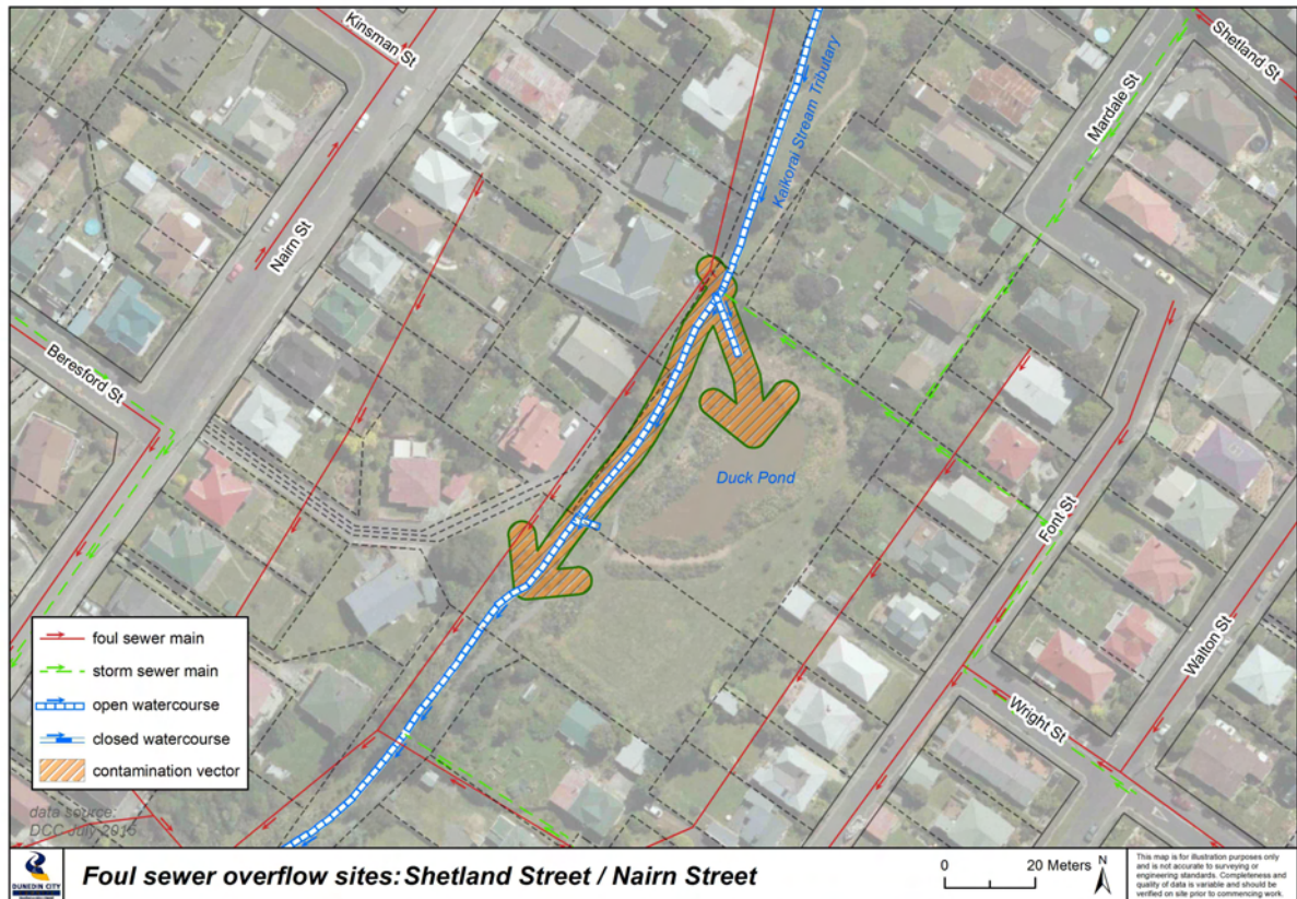
Figure 4. Aerial photograph detailing Kaikorai Valley wastewater network pipes (red lines) and the location of the Shetland Street / Nairn Street wastewater overflow (orange arrow) which discharges to a tributary of Kaikorai Stream (blue and white line).
