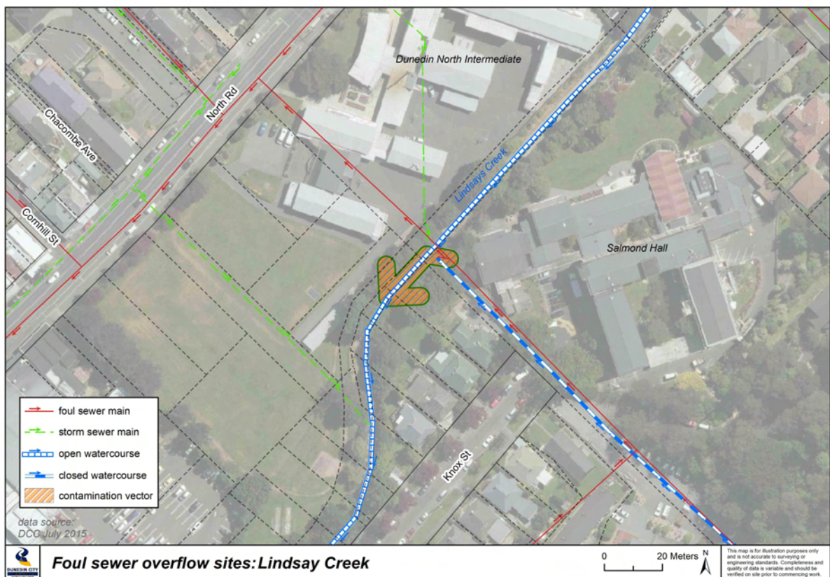
Figure 6. Aerial photograph detailing North East Valley wastewater network pipes (red lines) and the location of the Lindsay Creek wastewater overflow (orange arrow) which discharges to Lindsay Creek (curved blue and white line).
