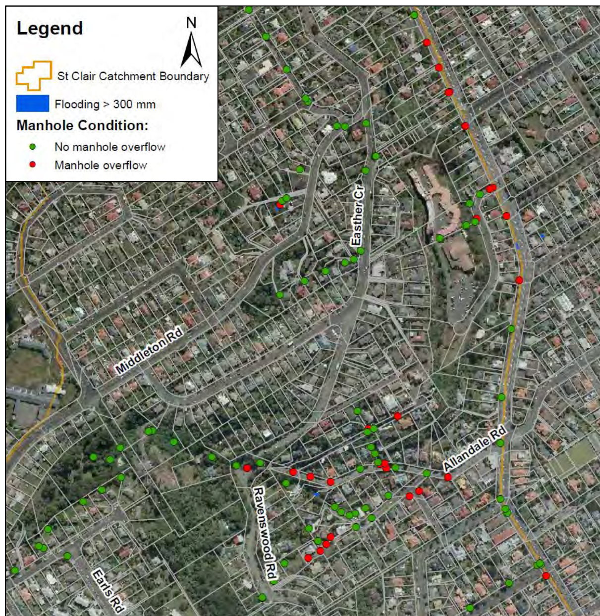
Figure 64: St Clair catchment potential habitable floor flooding during 1 in 50 year ARI rainfall event
