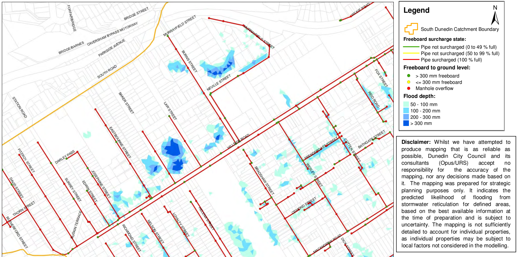
Figure 8-7: Predicted Flooding, Neville Street, Burns Street, Law Street and Baker Street, during a Current 1 in 50 yr ARI Rainfall Event
