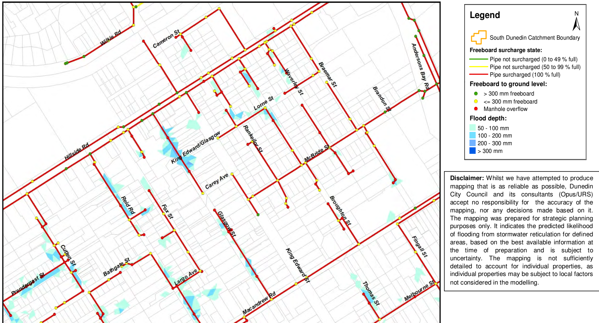
Figure 8-4: Predicted Flooding due to Hillside South Trunk Main Surcharging during a 1 in 10 yr ARI Rainfall Event (Current Land Use)
