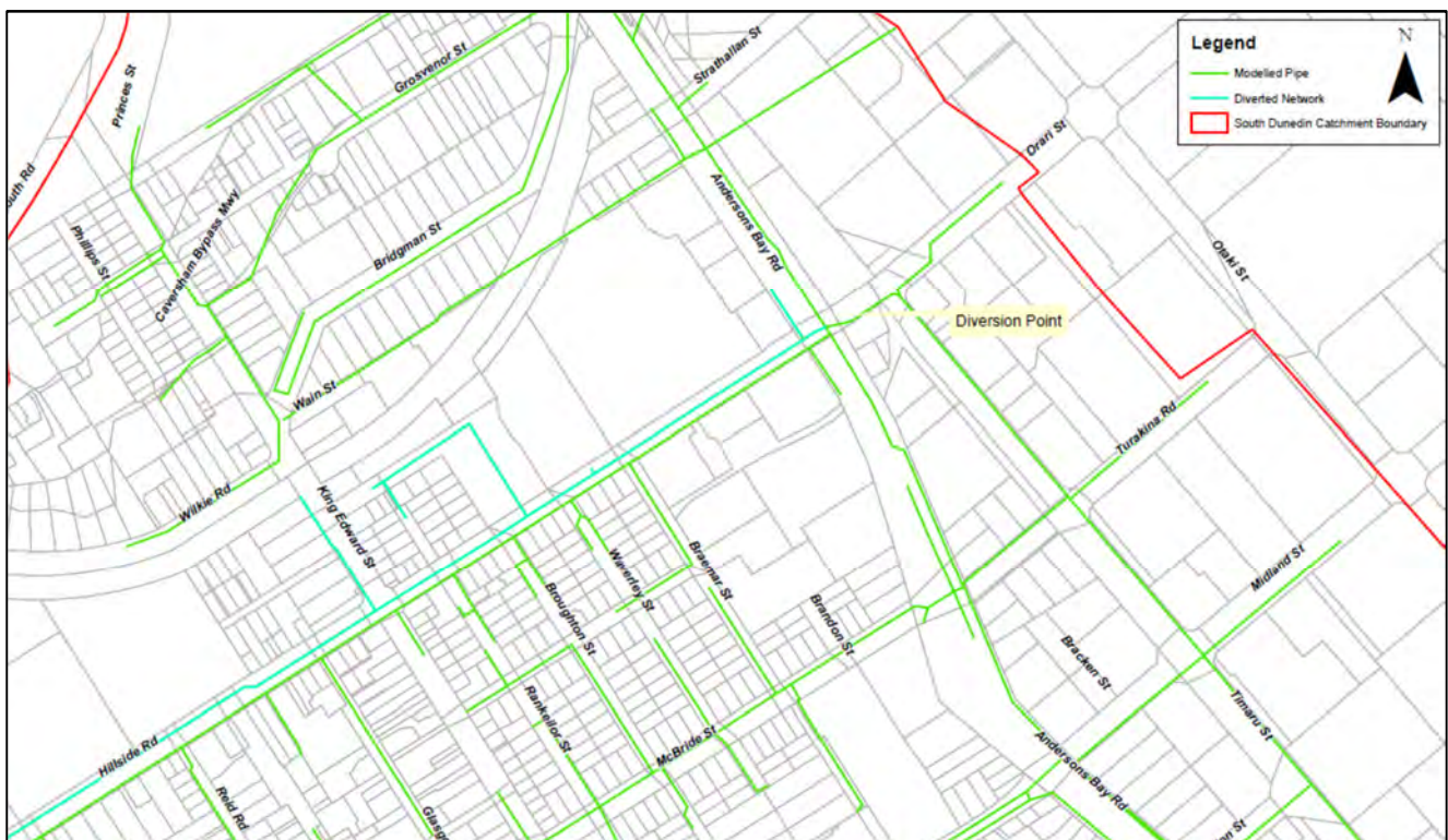
Figure 12-1: Modelled Diversion of Hillside Road Stormwater
