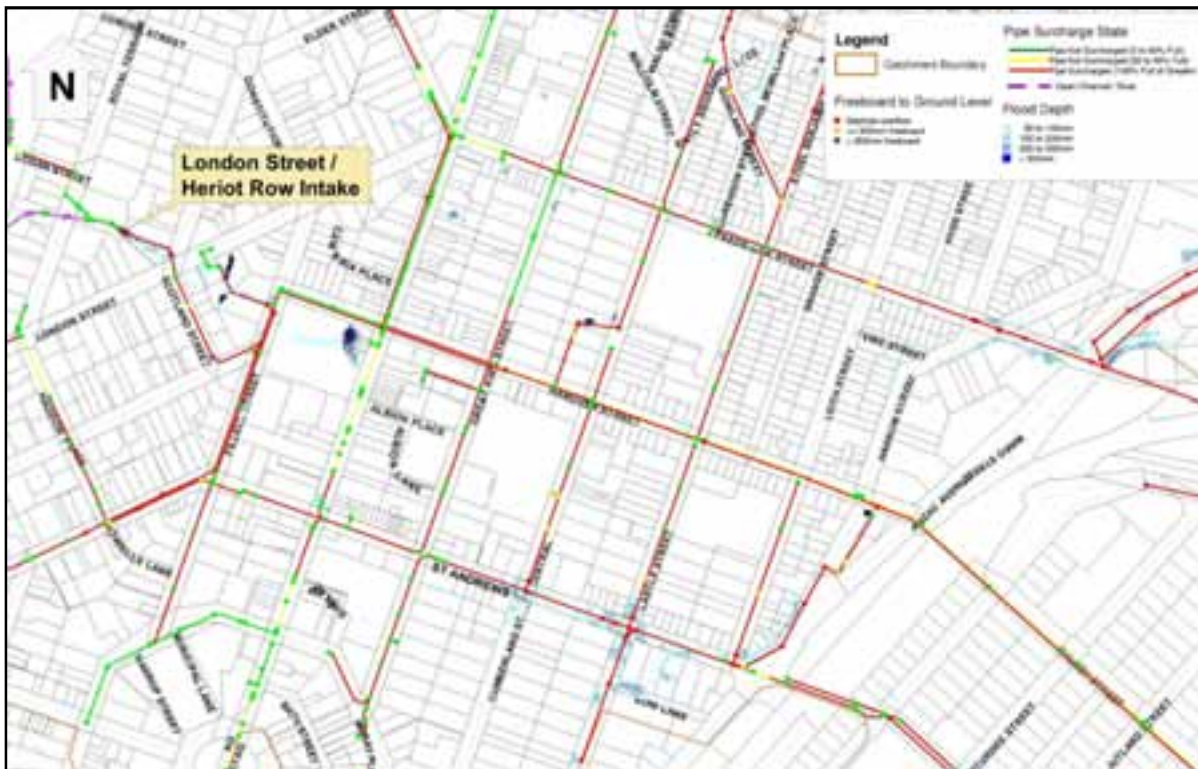
Figure 8-3: 2010 1 in 10 yr ARI Rainfall Event (Model Results) - London Street / Filleul Street / York Place / St Andrew Street
