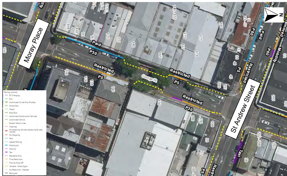
Figure 3: Existing kerbside restrictions – Farmers Block
